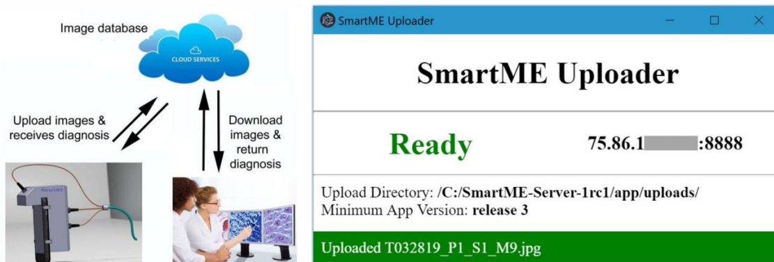
Figure 4-7: SmartME remote server
